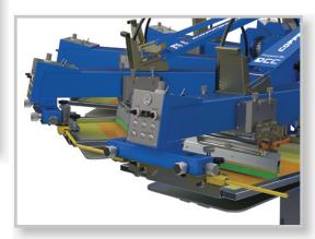
Individual mechanical heads lift for quick screen cleaning
